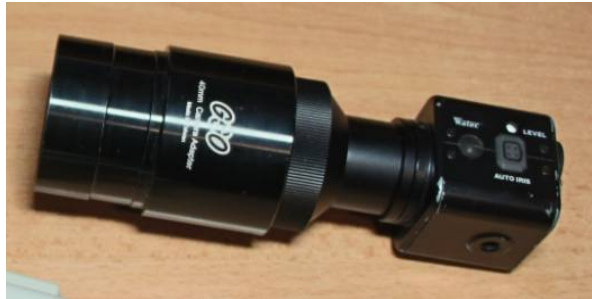
A highly rigid refractor setup with (L to R) 2" to T2 Adaptor with extension, T2 to C Adaptor with extension, Camera
