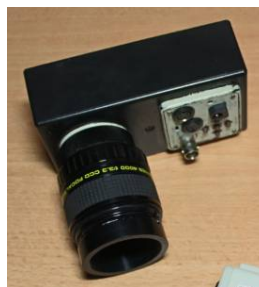
The Meade f3.3 Focal reducer is connected to a modified GStar-EX camera using a low profile C-T2 adaptor
