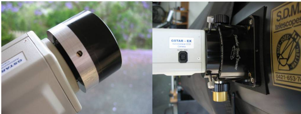
Machined 2" adaptor used to get focus on a 20" Dobsonian designed for visual work
